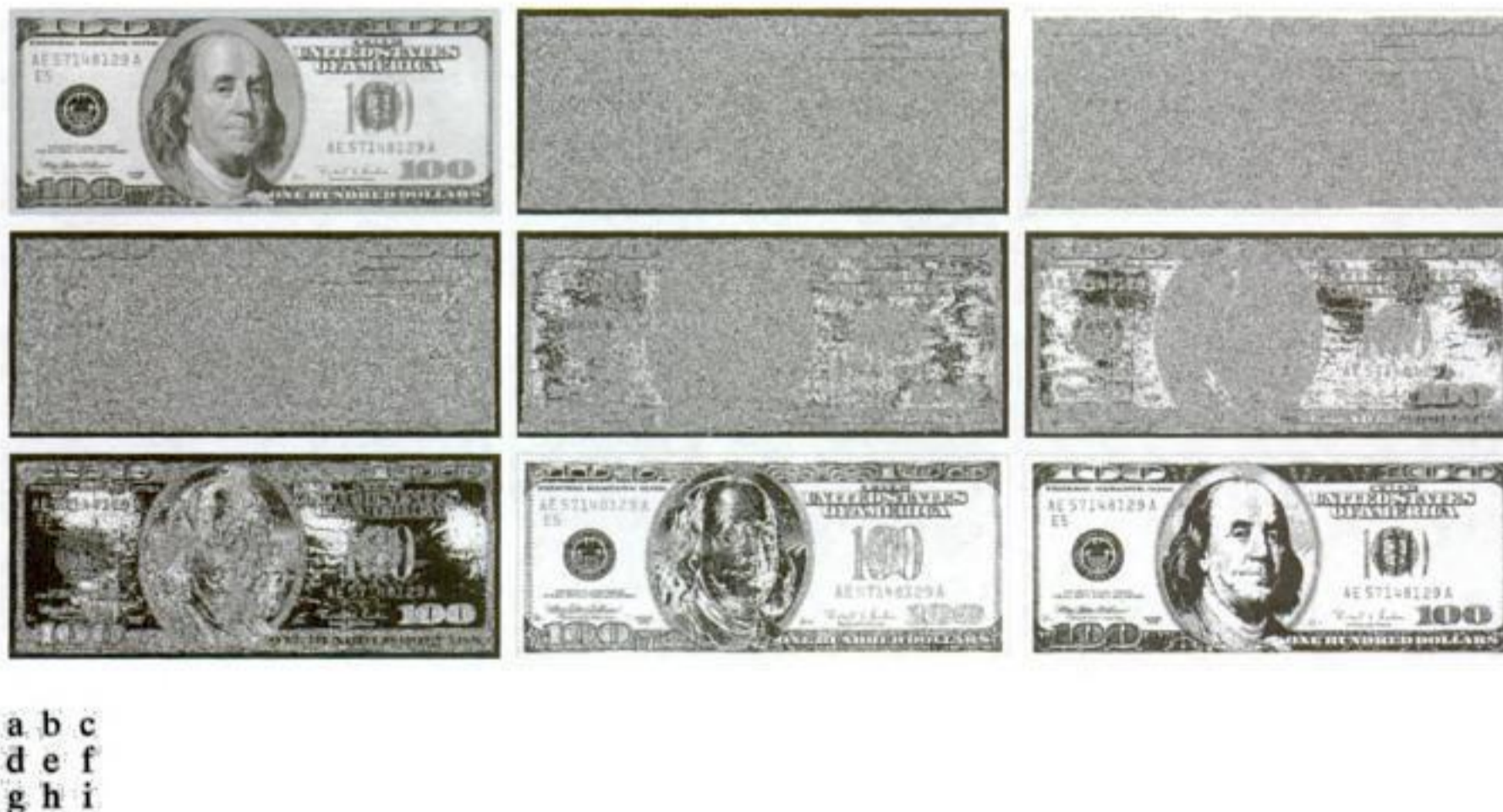
FIGURE 3.14 (a) An 8-bit gray-scale image of size 500 \times 1192 pixels. (b) through (i) Bit planes 1 through 8, with bit plane 1 corresponding to the least significant bit. Each bit plane is a binary image.
